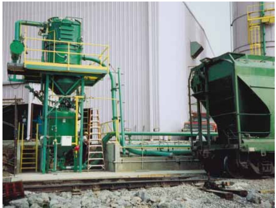
Shown above is a high density vacuum conveying system for unloading railcars.
