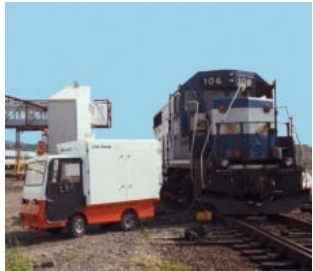
The Little Sandy portable locomotive sanding system conveys sand to the front of a locomotive that is in a remote location using a flexible hose and fill wand.
