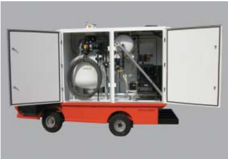
The Little Sandy portable locomotive sanding system with doors open, showing the transporter, air surge tank, air compressor, fill wand and convey hose. Everything is easily accessible for maintenance and enclosed for protection from outside elements.
