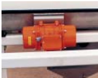
Vibrating hopper enhances gravity feeding of coarse materials.
