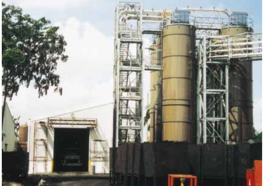
Shown above is an HDV 8000 vacuum system combined with a Dense Phase Full Line system that conveys carbon black to six storage silos.
