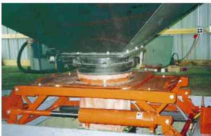
Shown above is a power boot lift in combination with an HDV 8000 vacuum unloading system directly connected to the hopper bottom of a truck.
