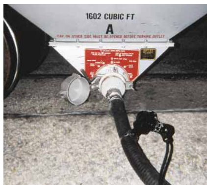
Shown above is a pickup pan and vacuum hose connected to a railcar in combination with an HDV 8000 vacuum unloading system for polyethylene pellets.
