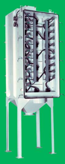
Back View showing access door to clean air plenum for inspection and maintenance of solenoid valves wired to a NEMA 12 enclosure.
