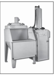
Cruncher bag compactor mounted to BagBuster bag breaker.
