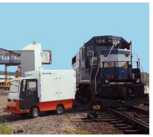
The Little Sandy portable locomotive sanding system conveys sand to the front of a locomotive that is in a remote location using a flexible hose and fill wand.
