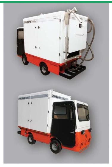
The Series 714 Model 100 Little Sandy portable locomotive sanding system is capable of delivering sand to locomotives at a rate of 3000 pounds per hour or more. The system is totally self sufficient and includes a dense phase Full Line Concept® pneumatic conveying system complete with an electric start powered air compressor, air surge tank, moisture separator and a programmable controller. Also included is a heavy-duty weatherproof enclosure with 20 feet of hose and an aluminum fill wand.
