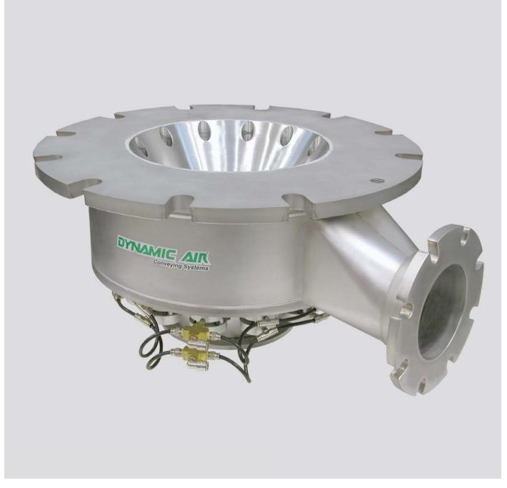
The Series 705 Blendcon<sup>®</sup> 12-port high capacity continuous blender is completely air operated with spring return pistons and single port supply
