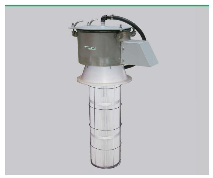
The Modu-Kleen® Series 725 top removal bin vent filter allows vented discharge air to be exhausted but prevents any outside atmospheric air from entering the storage silo or surge bin. This is ideal for venting storage bins and silos which contain hygroscopic materials that absorb moisture from the atmosphere. Materials such as granulated sugar and salt remain lump free and are handled much easier. The Modu-Kleen Series 725 bin vent filter fully meets the new OSHA requirements for confined
