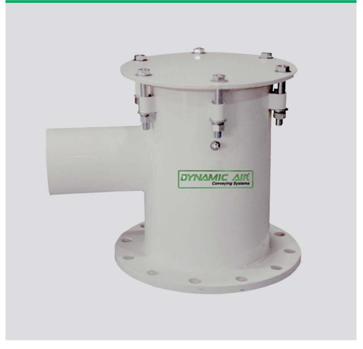
The Series 106 End Receiver by Dynamic Air Inc. allows the material conveyed to be discharged from the conveying line into a receiving bin, hopper or silo. The low profile design can be used on most materials conveyed and includes a unique rotating outlet for simpler, faster and easier installation. The heavy-duty construction is fabricated of either all mild steel, stainless steel or aluminum.
