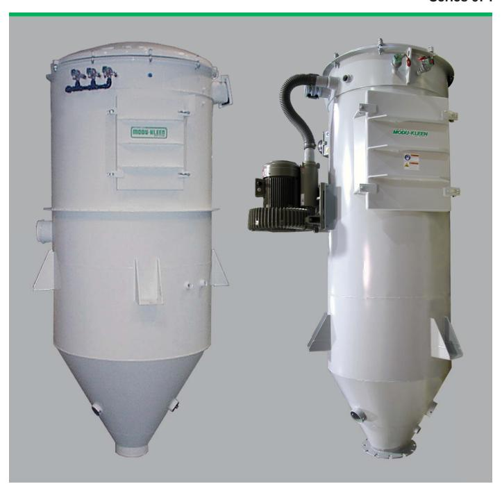
The Series 674 Vacuum Filter Receiver by Dynamic Air Inc. features a full vacuum rated housing, quick release cartridge filters or bag filters with included special wear resistant inlet fitting, inside grating for easier filter removal, vacuum rated discharge valve
