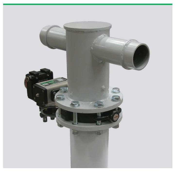
The Series 412 Valve Receiver from Dynamic Air Inc. allows material to be discharged from a conveying line with a full line of material. It includes a heavy duty housing with mounting flange and one (1) Posi-flate inflatable seat butterfly valve complete with air operator and solenoid valve. Construction is all mild steel as standard or optional stainless steel or aluminum.
