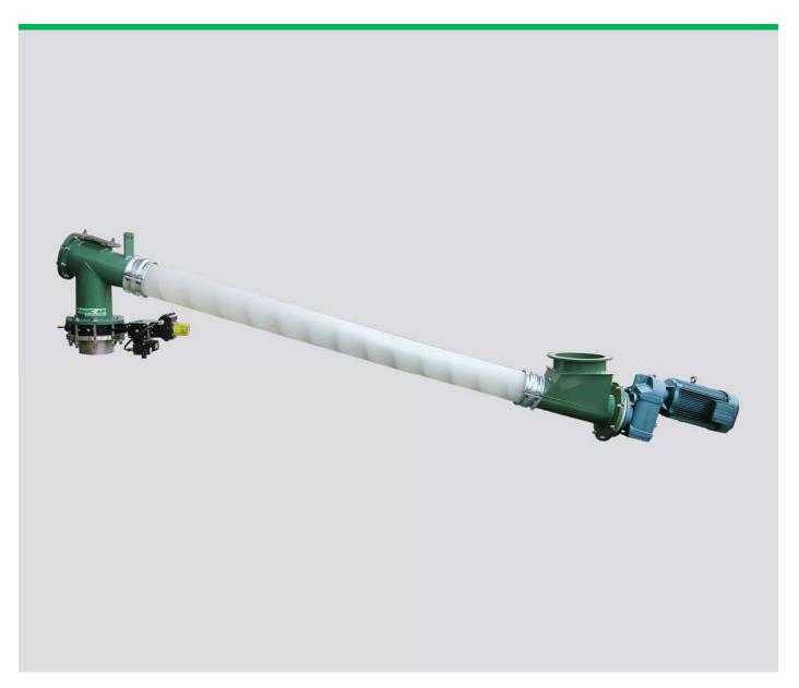
The ISO-LIFT™ flexible screw conveyor is used to convey almost any dry bulk solid material, including fine and dusty chemicals and/or dry powders, up to 80 feet horizontally as well as vertically. It is versatile with regard to the particle size, bulk density and moisture it can convey. In addition, the ISO-LIFT flexible screw conveyor is completely dust-tight and low in cost. Because the screw flighting is allowed to float inside the flexible tube of the ISO-LIFT
