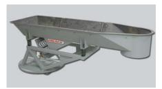
This STEDI-FLO Two-Mass Rotating Vibratory Feeder is used as a foundry charge feeder to charge scrap metal into a melting furnace. This feeder includes a special gear operated rotating base to feed two different furnaces as required. Also incorporated is a counterbalanced base to isolate the counteracting forces of the vibrating motor feeder and an abrasion resistant and easily replaceable liner.
