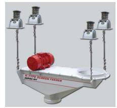
The K-Type Screen Feeder is a screen and feeder combination using a single or double deck screen with a brute force drive and a single electric vibrating motor. It is ideal for screening dry granular material from one inch down to 100 mesh particle size. The K-Type Screen Feeder can be flood fed and suspension or base mounted directly below any size surge hopper. The replaceable screen deck can be constructed of a 500 Brinell abrasion resistant steel
