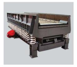
These EZ-WERK<sup>TM</sup> Foundry Shakeouts are used to separate sand from castings in iron foundries. They include counterbalanced bases to isolate counteracting forces. The finger decks, which are easily replaceable, are specially designed and fabricated of abrasion resistant steel to maximize the shakeout performance.
