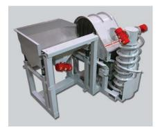
This Foundry Reclaim Unit uses a STEDI-FLO Vibratory Feeder to feed floor scrap from front end loaders onto a reclaim drum feeder. The drum feeder separates large particles such as steel rods, chaplets, etc from sand and steel shot. Any particles larger than ½ inch are fed into a collection hopper for remelting. Anything smaller than ½ inch is fed to a vibrating screen which separates anything larger than 50 mesh to a collection barrel.
