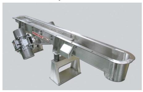
The STEDI-FLO™ Vibratory Screen Feeder is a screen and feeder combination using either a single, double or triple deck screen and a brute force drive with two electric vibrating motors. It is ideal for screening dry granular material from one inch down to 30 mesh particle size.
