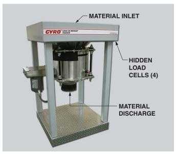
The GYRO Loss-In-Weight Feeder is both a loss-in-weight feeder and a bin discharger, all in one unit. Using the power of rotary vibration, it generates a pure gyratory motion to feed almost any granular material, irrespective of particle size or difficult handling characteristics. Also, a variable speed controller allows the GYRO Loss-In-Weight Feeder to achieve up to a 400 to 1 turndown ratio for faster feed rates and lower dribble feed rates for high accuracy weighing and batching.
