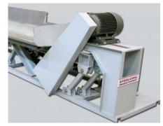
The STEDI-COIL<sup>™</sup> Vibratory Conveyor is used to convey either sand and castings together or sand and castings separately. This design also uses an abrasion resistant and replaceable conveyor trough and incorporates a heated and fully insulated trough to prevent sticky molding sand from adhering to the trough. Also included is a single but proven eccentric drive and a counterbalanced base to isolate the counteracting forces.
