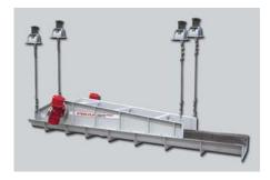
This STEDI-FLO Vibratory Feeder is installed in a midwestern iron foundry to convey fragile iron castings from an existing vibratory conveyor to an existing casting cooling vibratory conveyor at the rate of 240 castings per hour. The trough is made of abrasion resistant steel and designed for easy replacement. This application uses a suspension mount, which is required because of limited floor space.
