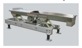
The STEDI-FLEX<sup>™</sup> Vibratory Conveyor is low in cost and simple in design and construction. It includes a counterbalanced base specially designed to isolate the counteracting forces produced in a conventional vibratory conveyor. It is available in any size width or length required and produced in both mild steel and stainless steel construction. A dust tight cover is optional.
