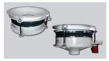
The GYRO™ Bin Activating Feeder produces 360 degrees of pure gyratory motion to positively and more reliably discharge granular materials from bins, storage silos and hoppers at any desired feed rate.
