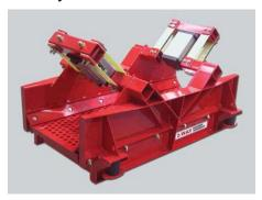
This Two-Way Air Operated Foundry Shakeout feeds foundry shakeout sand from a single vibratory feeder into two different directions. It uses two linear electric vibrators along with a replaceable abrasion resistant, steel shakeout deck. In addition, the feed rate is infinitely adjustable by controlling the air pressure and air volume as required.
