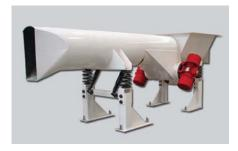
This STEDI-FLO Tubular Vibratory Feeder is designed to feed foundry sand to an existing bucket elevator from a surge hopper. It also includes a counterbalanced base to isolate the counteracting forces.
