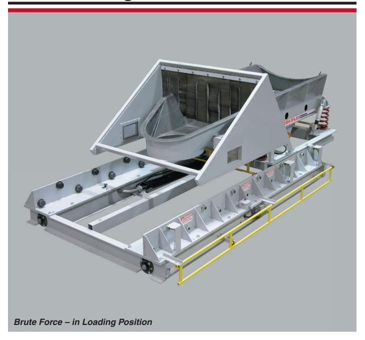
This Dynamic Air STEDI-FLO™ Vibratory Furnace Charge Feeder is used by an aluminum foundry to charge aluminum scrap into an electric melting
