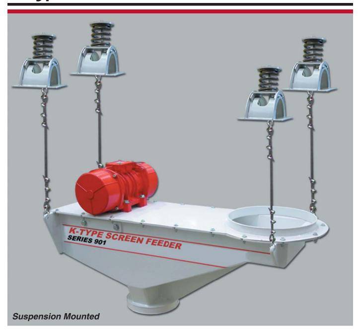
The Dynamic Air K-Type Screen Feeder is a screen and feeder combination using a single or double deck screen with a brute force drive and a single electric vibrating motor. It is ideal for screening dry granular material from one inch down to 100 mesh particle size. The K-Type Screen Feeder can be flood fed and mounted directly below any size surge
