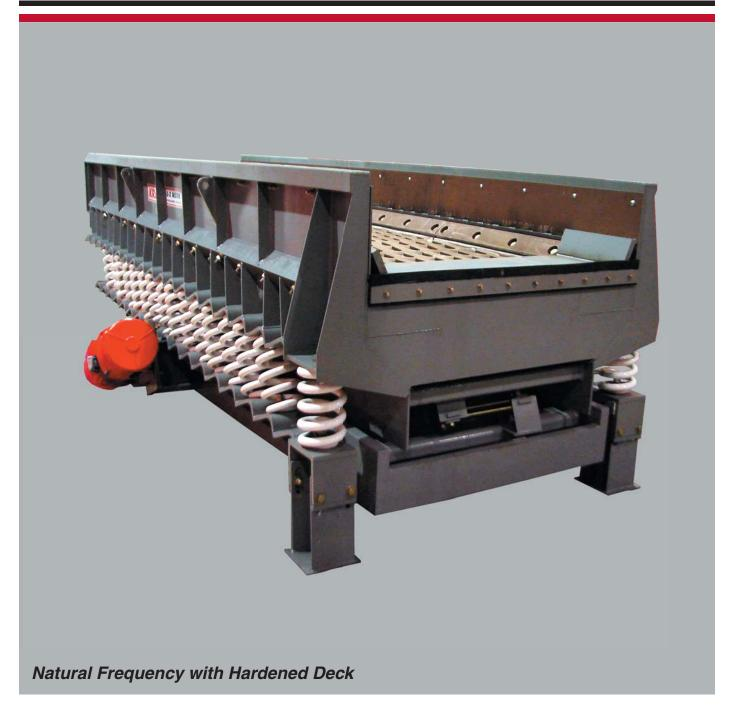
This EZ-WERK™ Vibratory Shakeout by Dynamic Air is used to separate sand from castings in an iron foundry. It also includes a counterbalanced base to isolate the counteracting forces. The deck is a specially
