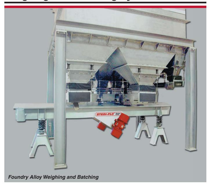
This Weighing and Batching System by Dynamic Air uses multiple L-Type Vibratory Feeders to feed individual ingredients onto one STEDI-FLO™ Vibratory Feeder. The STEDI-FLO Vibratory Feeder is mounted on four load cells, one under each spring support leg. Individual ingredients are weighed in succession until the weighed
