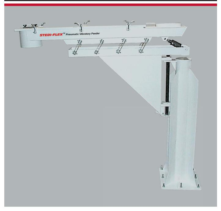
This Dynamic Air STEDI-FLEX<sup>™</sup> Vibratory Feeder is powered by a vibrating linear air motor and is used to convey foundry sand to two (2) different core sand mixers from a single surge hopper which is fed by a dense phase pneumatic conveying system.
