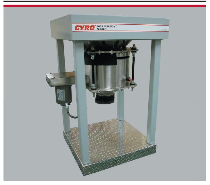
The GYRO™ Loss-In-Weight Feeder is both a loss-in-weight feeder and a bin discharger, all in one unit. Using the power of rotary vibration, it generates a pure gyratory motion to feed almost any granular material, irrespective of particle size or difficult handling characteristics. Also, a variable speed controller allows the GYRO Loss-In-Weight Feeder to achieve up to a 400 to 1 turndown
