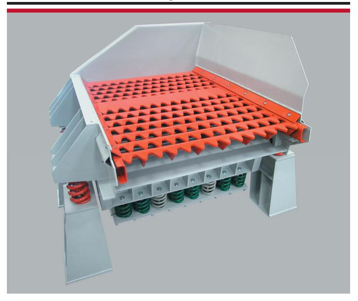
This Series 923 EZ-WERK™ Vibratory Shakeout by Dynamic Air is a natural frequency vibratory shakeout which handles up to 60 inch square by 30 inch high molds, weighing up to 10,000 pounds, at a rate of one every fifteen minutes. It uses the proven AR hardened finger deck for longer life. The molds are dumped from a mold dump onto the side of the shakeout to meet
