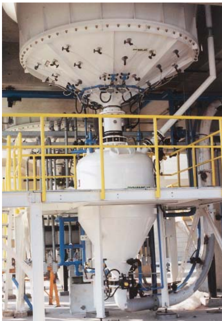
Dense phase transporter with a Vibra-Jet® bin discharger conveying detergent.
