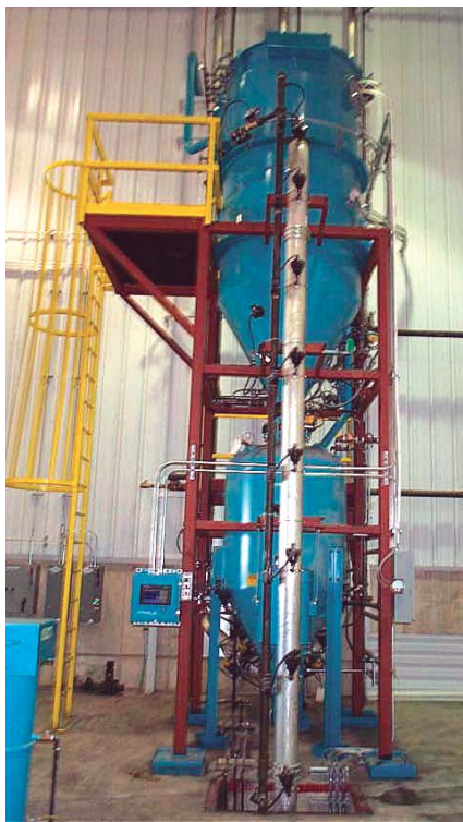
HDV™ high density vacuum Full Line Concept® conveying system located inside a truck unloading building.
