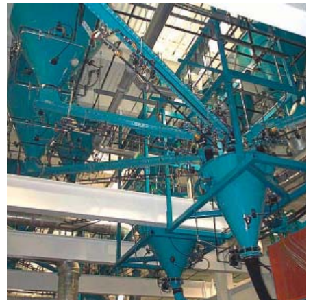
Dyna-Slide™ high precision feeders convey material from 200 cu. ft. (6 cu. m) surge bins to weigh hoppers.
